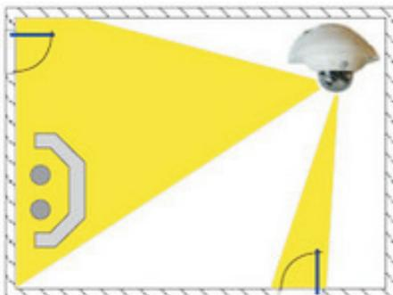
Two freely positionable camera modules
